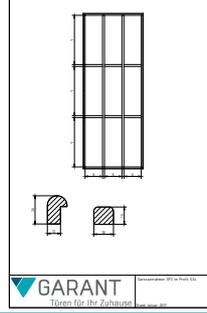
The diagram shows a vertical door frame with three vertical bars and two horizontal bars. Below the frame are two small icons: one showing a cross-section of the frame and another showing a detail of the bar. At the bottom left is the GARANT logo and the text 'Türen für Ihr Zuhause'. At the bottom right, it says 'Sprossenrahmen SP2 in Profil S34'.
