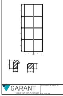
The diagram shows a vertical door frame with two vertical bars and two horizontal bars. Below the frame are two small icons: one showing a cross-section of the frame and another showing a detail of the bar. At the bottom left is the GARANT logo and the text 'Türen für Ihr Zuhause'. At the bottom right, it says 'Sprossenrahmen SP1 in Profil S34'.
