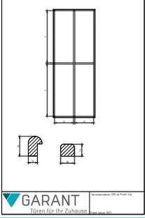
The diagram shows a vertical door frame with two vertical bars and one horizontal bar. Below the frame are two small icons: one showing a cross-section of the frame and another showing a detail of the bar. At the bottom left is the GARANT logo and the text 'Türen für Ihr Zuhause'. At the bottom right, it says 'Sprossenrahmen SP0 in Profil S34'.
