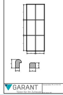
The diagram shows a vertical door frame with two vertical bars and three horizontal bars. Below the frame are two small icons: one showing a cross-section of the frame and another showing a detail of the bar. At the bottom left is the GARANT logo and the text 'Türen für Ihr Zuhause'. At the bottom right, it says 'Sprossenrahmen SP4 in Profil S34'.
