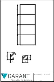
The diagram shows a vertical door frame with two vertical bars and four horizontal bars. Below the frame are two small icons: one showing a cross-section of the frame and another showing a detail of the bar. At the bottom left is the GARANT logo and the text 'Türen für Ihr Zuhause'. At the bottom right, it says 'Sprossenrahmen SP10 in Profil S34'.
